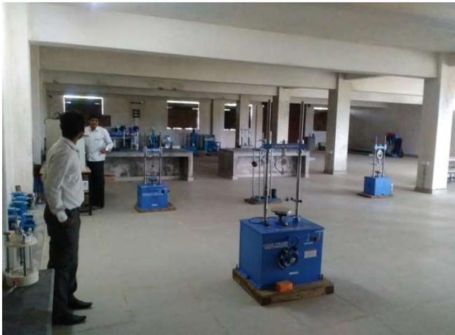
The soil properties, its changing behavior are studied here. Students perform consolidation test, core cutter test, standard and proctor compaction, unconfined compression test, tri axial compression test and many more.
