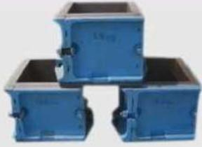
Fig: Standard cube mould
