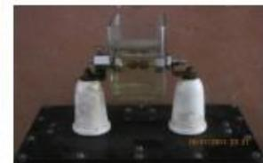
Fig.1: Portable oil testing set
